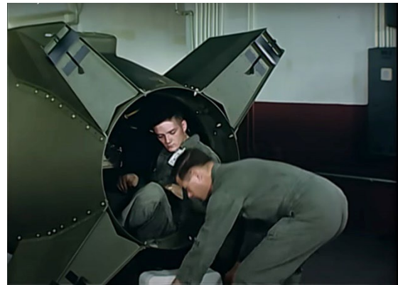
Left: MK 7 nuclear bomb with related test equipment. Right: Many nuclear weapons tasks required hands, arms, head or entire body to be inside. Images: SN Lab, “Early Nuclear Safety” video.
