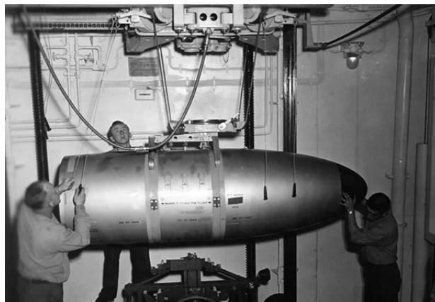
MK7 Bomb (warhead without rear section) - Hoisting operation for maintenance tasks on a ship. The MK7 could be carried by Navy and AF aircraft. Photo credit: unknown.
